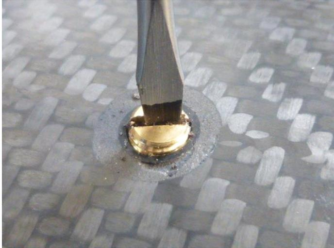
Screw the grub screw into the fitting until the pen mark is level with the bottom of the hull. The mark on the screwdriver shaft is just visible in the photo below. The fitting is now fully inserted.
