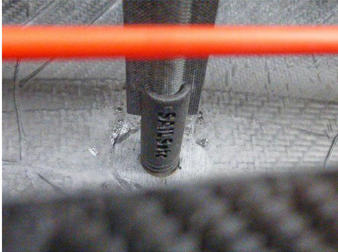
Shorten the Tube J so that the 12 mm diameter section of the fitting just fills the hole in the hull bottom.
