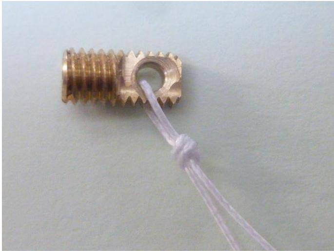
The grub screw will be inserted until its upper end is still just engaged with the thread. Mark your screwdriver to show where this will be.
