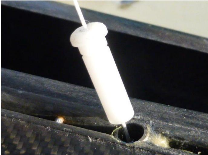
Tie the ring securely as close as possible to the deck. Seal the knot with cyanoacrylate glue and trim off excess line.
