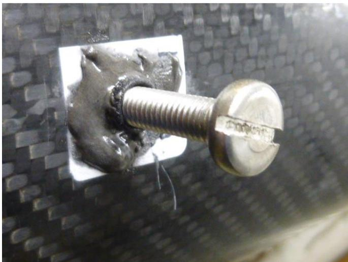
Clean up excess resin and form the remainder into roughly the shape required. Allow to cure until tacky but still malleable – between 1 and 2 hours depending on temperature and speed of cure.
