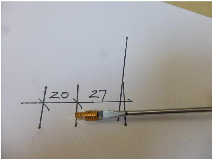
Pass the line up the tube and screw the grub screw into the thread.
