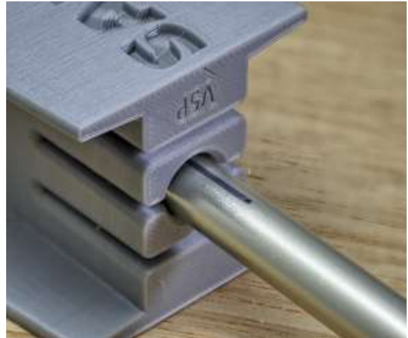
Figure 3. Axis of tube symmetry aligned with track vertical plane
