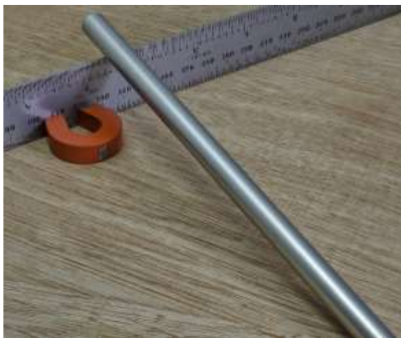
Figure 2. Checking for straightness and identifying the axis of symmetry
