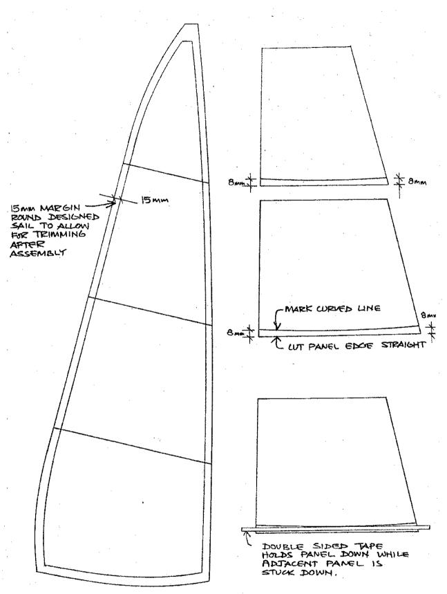
Pattern for the sail should allow a 15 mm margin around all edges. Mark the panel edges with the desired seam shape.
