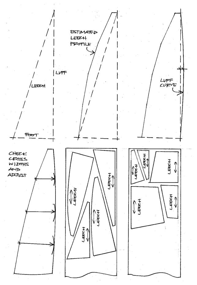
Set out the profile of the sail, mark the estimated leech shape, add the luff shape, then check the cross widths and adjust. The leech of all sails and panels should be aligned with the warp of the cloth.
