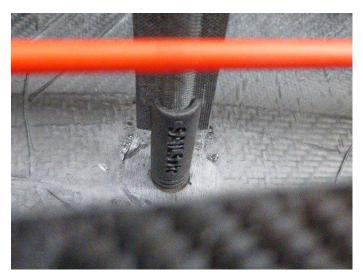
Shorten the Tube J so that the 12 mm diameter section of the fitting just fills the hole in the hull bottom.
