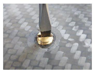
Screw the grub screw into the fitting until the pen mark is level with the bottom of the hull. The mark on the screwdriver shaft is just visible in the photo below. The fitting is now fully inserted.
