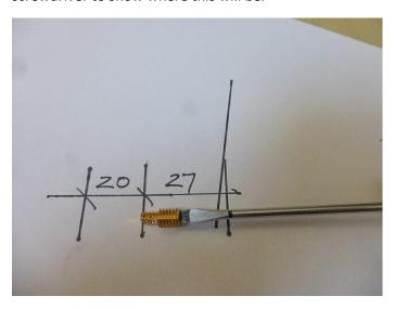
Pass the line up the tube and screw the grub screw into the thread.
