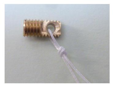
The grub screw will be inserted until its upper end is still just engaged with the thread. Mark your screwdriver to show where this will be.
