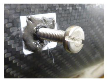
Clean up excess resin and form the remainder into roughly the shape required. Allow to cure until tacky but still malleable – between 1 and 2 hours depending on temperature and speed of cure.
