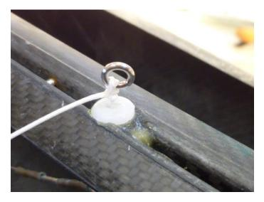
When the rig is added and tensioned you can use the grub screw to lower the ring until it just clears the deck.
